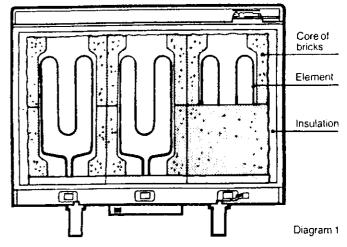
In the morning, when the core is at its hottest, the amount of heat being transmitted through the insulation and emitted as radiant heat is at its greatest, and the heater feels hot over most of its outer surfaces. Diagram 2.
